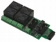
Relay Board - 4 is a Quad 10A SPDT relay board with logic level drivers. It is suitable for use with TowerMan, TC-64, LNCP, or other logic output devices. It requires 12V auxiliary power to drive the relay coils. Auxiliary power is optically isolated from the logic inputs for double isolation. LED indicators for each relay make it easy to monitor activity.
