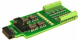
This 8 input board is used when a non-isolated source of voltage needs to be monitored and input to the TowerMan. One example would be to monitor the DCC voltage on a set of points to determine the position of a turnout without using auxiliary contacts.
