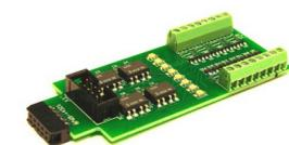
This 8 input board is used when a non-isolated source of voltage needs to be monitored and input to the Tower LCC. One example would be to monitor the DCC voltage on a set of points to determine the position of a turnout without using auxiliary contacts.
