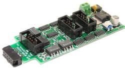
The SMD-8 board contains 8 individual, optically isolated, H-Bridge drivers. This allows the board to be powered from any supply between 9 Volts and 27 Volts. It is primarily designed to drive stall motor turnout machines such as those found in Tortoise® and Switchcraft® machines . Do not exceed 20VAC or 27VDC at the power input.
