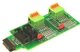
This board is a convenient way to convert from 10 pin ribbon cable to compression terminals. It may be used for inputs or outputs, and includes pads for mounting resistors such as may be required for connecting LEDs used for direct drive signals or panels.
