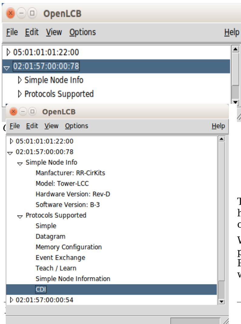
**Select** the node that you desire to configure and click on its arrow to open it. This will open up further options for that node. In this example there is an option for 'Simple Node Information' and a list of 'Protocols Supported'.
