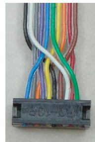
conversion at the end of your cable it will allow the SignalMan to connect to the TAB-2 or TAB-3 boards for solderless plug connections to your Tortoise® machines. (the blue and green connections are optional for the TAB-2, but supply the lamp circuit on the TAB-3.)
