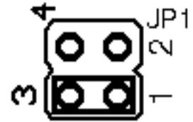
For use on a stand alone bus the Master Mode must be enabled by manually writing to CV 112 before removing the JP1 1-3 jumper.
