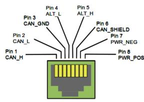
LCC power is supplied between Pin 7 and Pin 8. Power can be from +12VDC to +27VDC. The RR-CirKits LCC Power-Point delivers approximately 15VDC to the bus.
