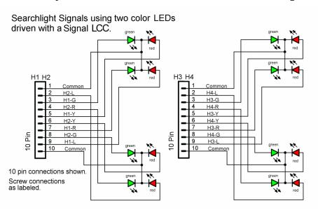
Signal LCC-32H Signal Wiring for two color (3 lead R/G) LEDs
