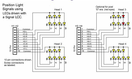
This shows the simplest wiring option for position light signals. The advantage of serial connection is that all LEDs receive the same current and will show with equal brightness. LEDs are current, not voltage operated devices, and even units from the same batch will often show with different brightnesses when connected in parallel.
