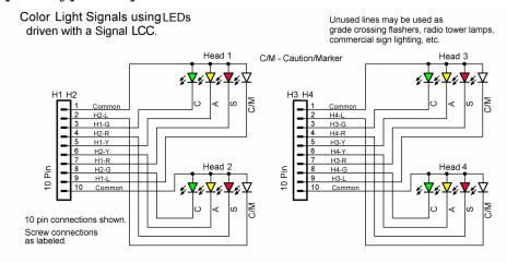
Signal LCC-32H Signal Head Wiring for Color Light Signals.
