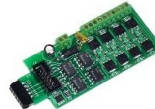
**Single Coil Solenoid Driver - 8** The SCSD-8 Output Module is designed to drive individual solenoid coils or other high voltage high power devices. Normally the input voltage should not exceed 35VDC. The SCSD-8 board is optically isolated from the driving circuitry to protect the TC-64 or other control device from the high power outputs.
